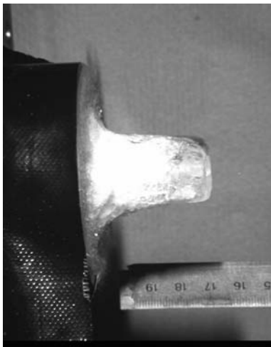
Fig. 2 Deformation and failure of ice cylinder projectile impacting load cell at 97.2 m/s
